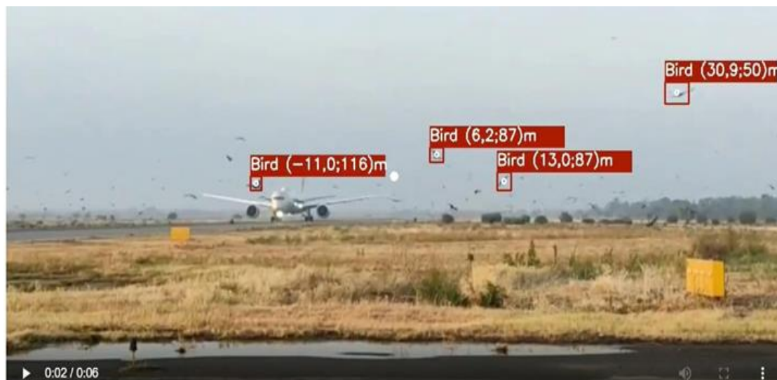
Figure 7. Object Detection with x,y,z coordinate with respect to camera
