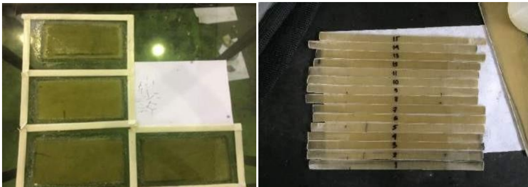
Figure 3. Hand Lay Up Specimens and Specimen Cuts
