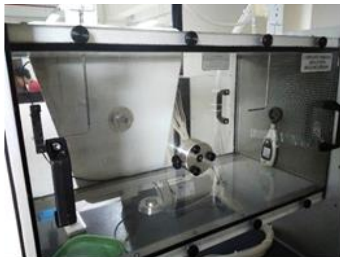
Figure 2. Anemometer inside the test section
