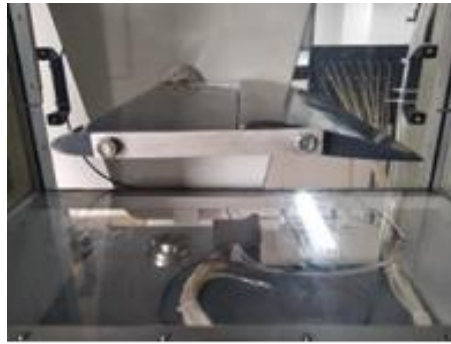
Figure 4. Tandem wing with NACA 0012 profile
